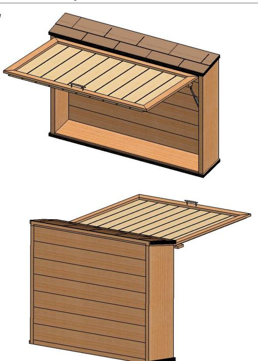
Install the asphalt shingles on the top of the cabinet following the manufacturers instructions. Use 1-1/4" Roofing Nails to secure the shingles to the top of the cabinet. The shingles will help the cabinet to shed water. Sand thoroughly and paint or stain as desired. Next install screw eyes at the top of the cabinet and the bottom of the door as shown.
