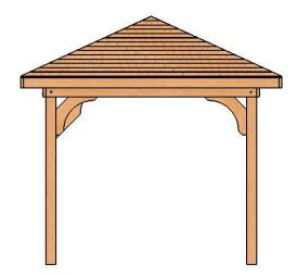
Field measure and cut  $2 \times 4$ 's to go around the roof as shown. Put one row around the very bottom of the roof. Place the top row about 3-1/2" below the peak of the roof. Place a row around the center of the roof spaced evenly between the top and bottom rows. You will screw the roof sheeting to these  $2 \times 4$ 's.
