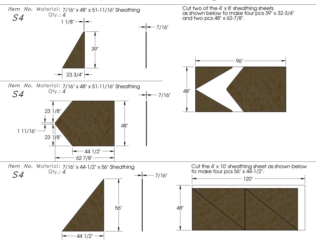
Install the roof sheeting as shown below making sure that each seam is centered on a rafter. Fasten to the rafters with 2" wood screws.
