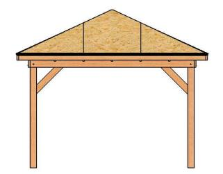
Cover the roof with roofing underlayment and fasten to roof with staples per manufacturers instructions.
