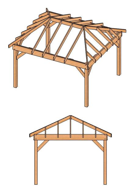
Install the last four hip rafters (Item # 14) on the front and rear of the gazebo frame as shown below. Fasten to the frame and end rafter assembly using 3" wood screws.
